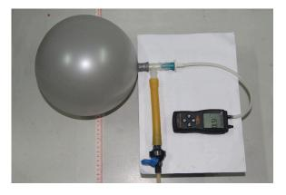
As is shown in the figure, a T-pipe connects the balloon, a manometer and a valve. A scale is placed to read the radius and pressure is obtained by manometer. The balloon is inflated at first to certain size, and the experiment starts as it deflates.
